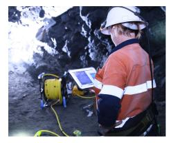
Once in the void it is capable of measuring the three-dimensional shape of the void with full 360° coverage with a range of up to 150 metres. All points collected are displayed in real-time in 3D view with the option of including existing models or data sets on-screen during collection.
